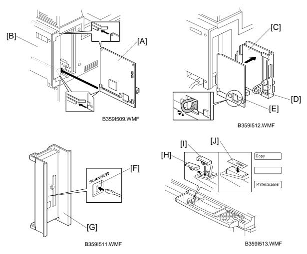
13. Install the scanner controller board [A] in the third slot from the right of the expansion box [B].
